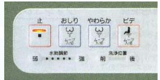
Electronic washlet toilet controls
